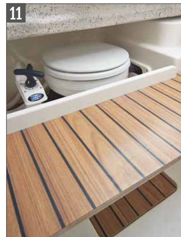
11 Cabin with concealed sea toilet
